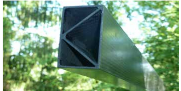
Longitudinal beam (cross section 50mm x 80mm) from 2,5 mm CFS ® - material
