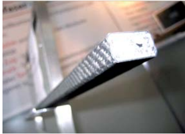
A 2 x 3 cm CFS bar made from granite is completely encapsulated and stabilized by a 1 mm carbon fibre laminate: high stiffness but flexible and with a consistent length across a wide temperature
